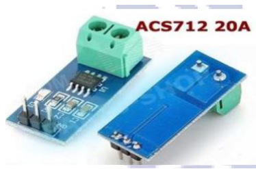
Gambar 1 Sensor Arus ACS 712
