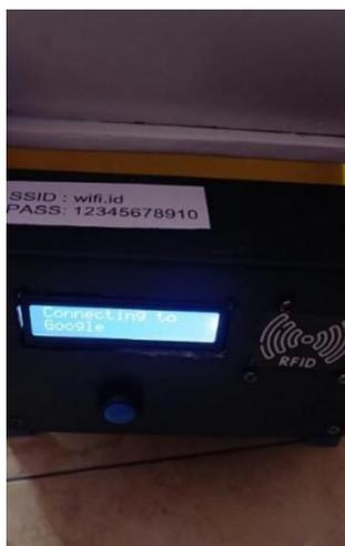
Fig. 6 Esp32 testing with Wi-Fi connection
