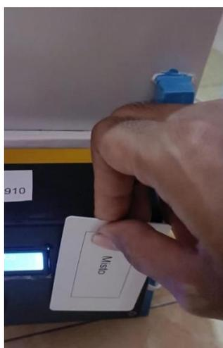
Fig.8 Card Testing with RFID-RC522 sensor
