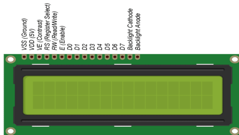
Figure 4. 16×2 LCD with interfacing comments.
