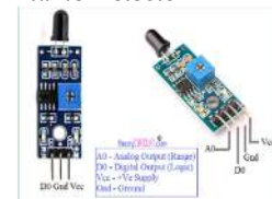
Gambar 5 Sensor IR Flame Detector (Sumber : https://theorycircuit.com/arduino-flame-sensor-interface/ )
