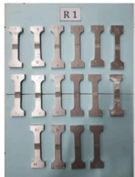
Gambar 9. Spesimen uji Tarik ASTM B 557M – 02a
