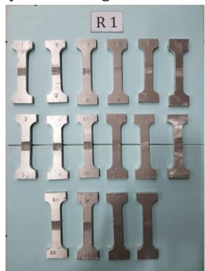
Gambar 9. Spesimen uji Tarik ASTM B 557M – 02a
