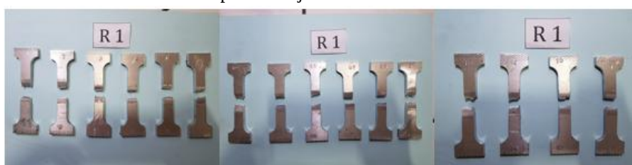
Gambar 10. Sampel patahan spesimen uji Tarik ASTM B 557M – 02a
