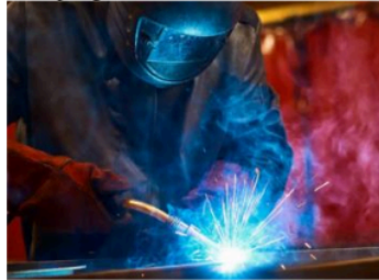
Gambar 3. Proses Pengelasan Metal Inert Gas (MIG)
