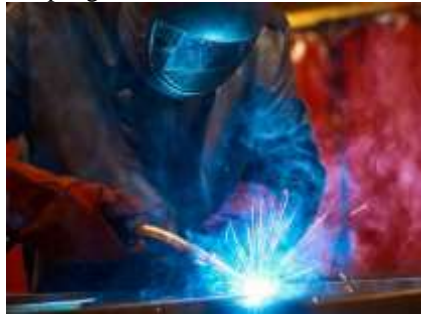
Gambar 3. Proses Pengelasan Metal Inert Gas (MIG)
