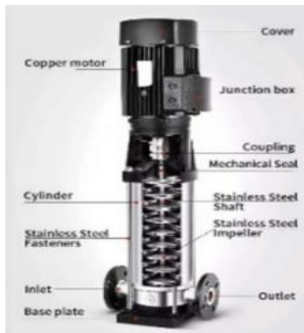
Gambar 3 Pompa Jockey Tipe CR Vertical Multistage Centrifugal
