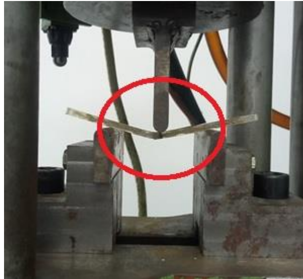
Gambar 16. Proses uji bending
