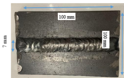
Gambar 6. Hasil Pengelasan Metal Inert Gas (MIG)
