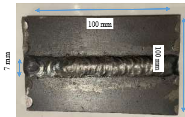
Gambar 7. Hasil Pengelasan Metal Inert Gas (MIG)
