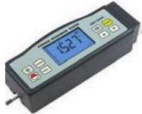
Gambar 10. Surface Roughness Tester
