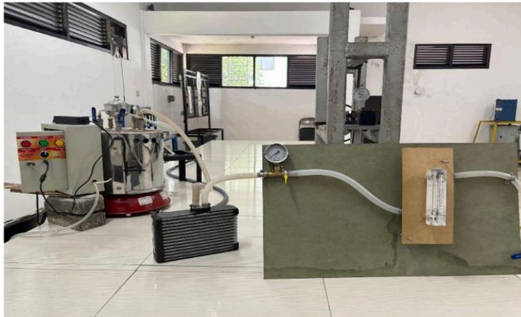
Gambar 2. Alat Uji Kondensor
