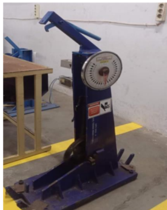
Gambar 9. Mesin Uji Impact Charpy Test 16
