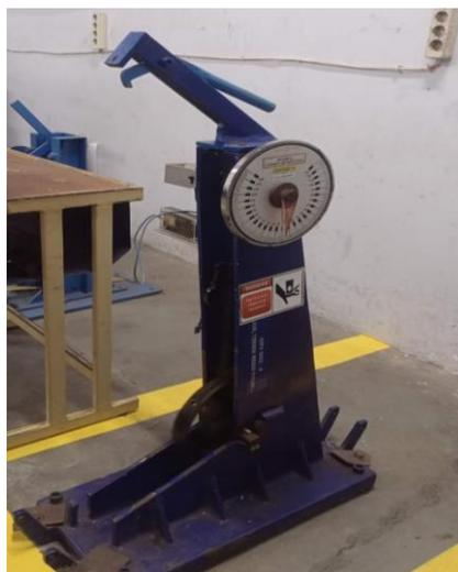
**Gambar 9.** Alat Uji *Impact Charpy Test*
