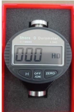
Gambar 10. Alat Uji Kekerasan Shore Durometer Digital
