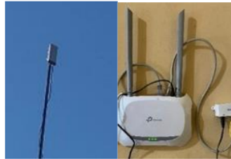
Gambar 8. Pemasangan Router Penerima (receiver) ke router TP-Link
