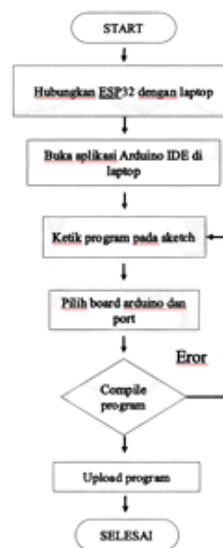
Gambar 2.5 Flowchart Software Arduino
