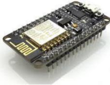
**Gambar 4.** NodeMCU ESP8266
