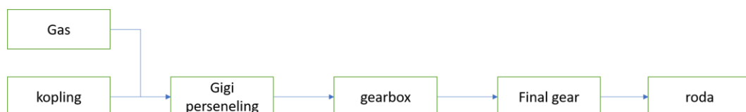
Gambar 2. Blok Diagram Pengoperasian Motor Secara Manual [2]
