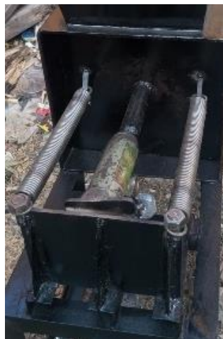
Gambar 5. Hasil erection piston pres
