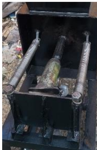
Gambar 5. Hasil erection piston pres
