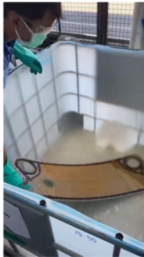
Gambar 3. Proses Perendaman Plat And Gasket Heat Exchanger
