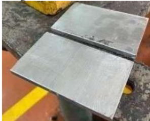
Gambar 11. Plat aluminium aa6061-t651
