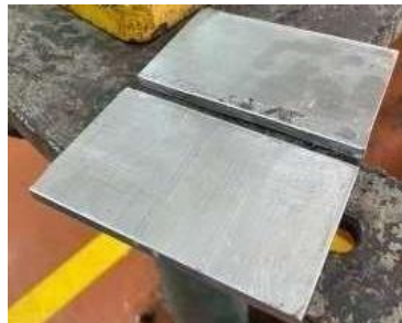
Gambar 11. Plat aluminium AA6061-T651
