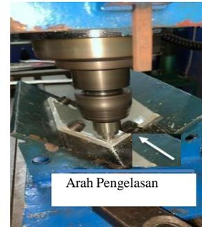
Proses *friction stir welding*
