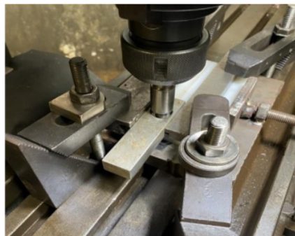
Gambar 1. Proses pengelasan FSW
