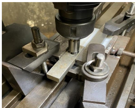
Gambar 1. Proses pengelasan FSW
