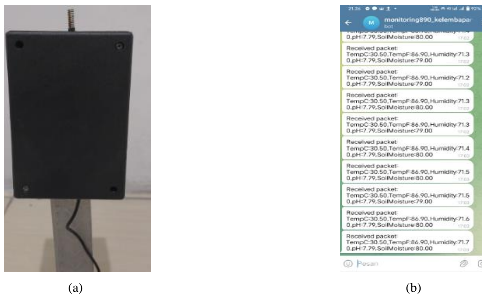
Gambar 5. (a)Alat receiver; (b) hasil pembacaan sensor
