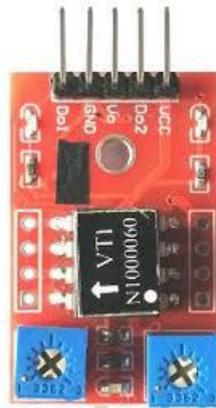
**Gambar 5.** Tampilan Sensor Axis Module SCA60C
