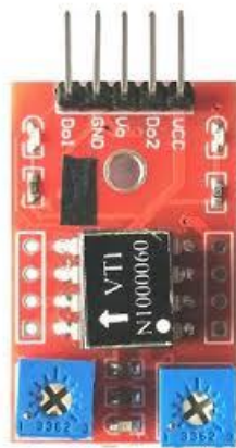
Gambar 5. Tampilan Sensor Axis Module SCA60C
