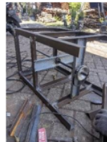
Gambar 3. Proses Perakitan As Poros dan Rumah Bearing
