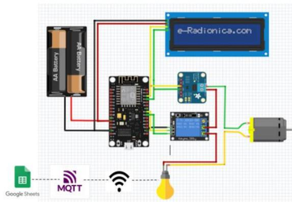
**Gambar 8.** Rangkaian sistem monitoring kendali beban
