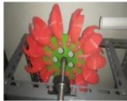
Gambar 1. Turbin Tipe Pelton
