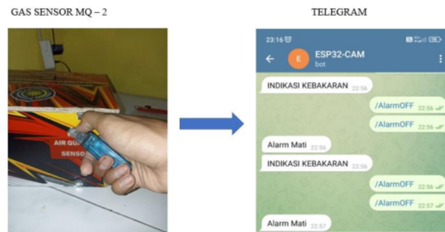
Gambar 4. Pengujian sensor Gas MQ – 2
