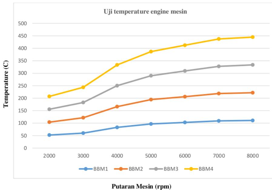
**Gambar 6.** Grafik temperature engine mesin
