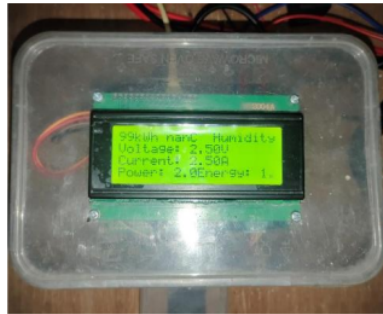
Gambar 7. Tampilan LCD I2C 20x4
