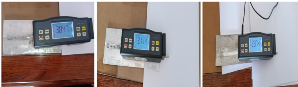
Gambar 7. Hasil uji kekasaran : (a) specimen 1 (b) specimen 2 (c) specimen 3
