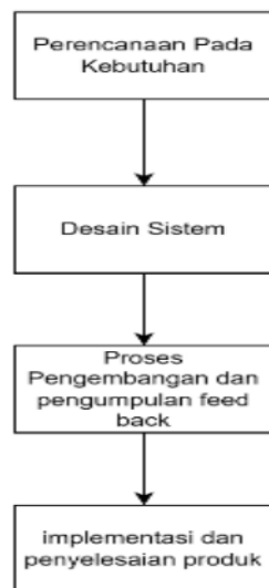
Gambar 1. Tahapan Rapid Application Development (RAD)
