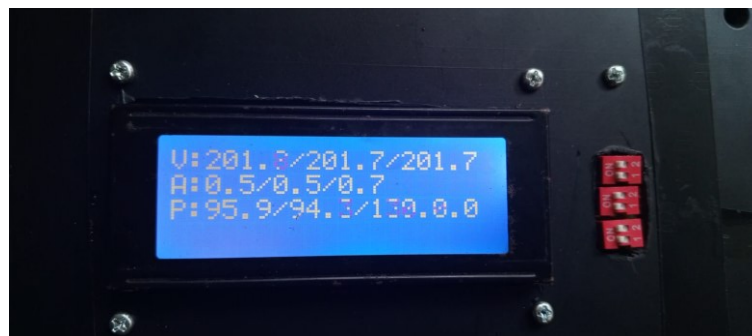
Gambar 7. Tampilan LCD I2C 20x4
