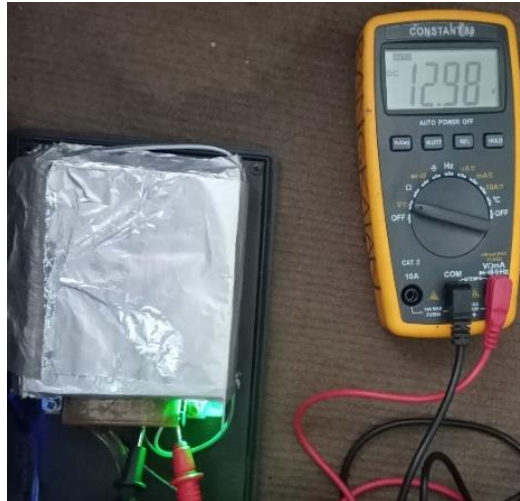
Gambar 9. Pengujian power supply
