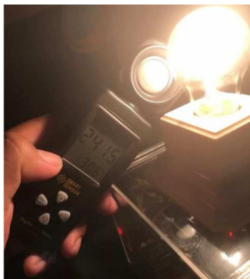
Figure. 13 Measurement using a lux meter
