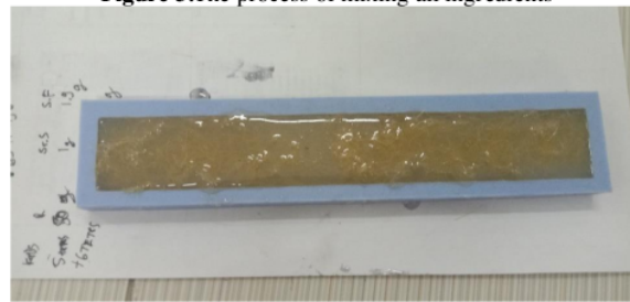
Figure 4. The material is poured into the mold
