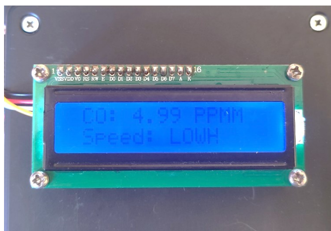
Gambar 7. Tampilan LCD I2C 16x2 saat nilai CO <10PPM
