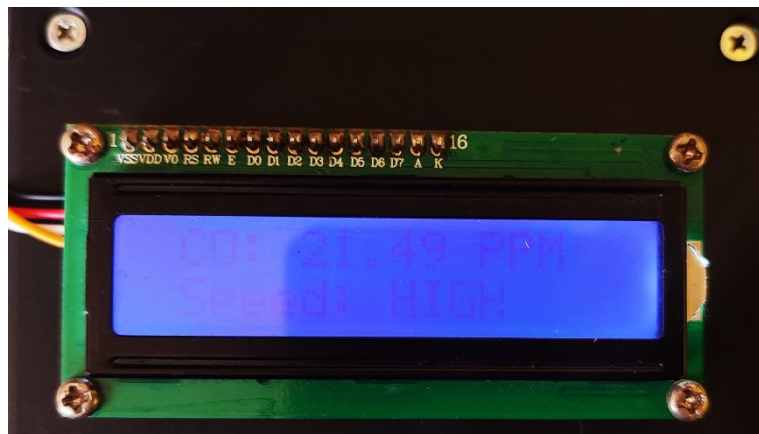
Gambar 9. Tampilan LCD I2C 16x2 saat nilai CO <21PPM
