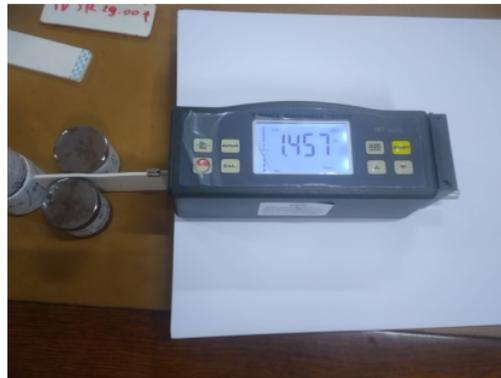
**Gambar 14** Alat Uji Kekasaran Permukaan (Surface Roughness Tester ( $\mu\text{m}$ ))
