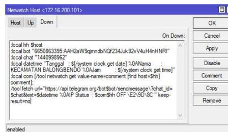
Gambar 4. Script down netwatch mikrotik
