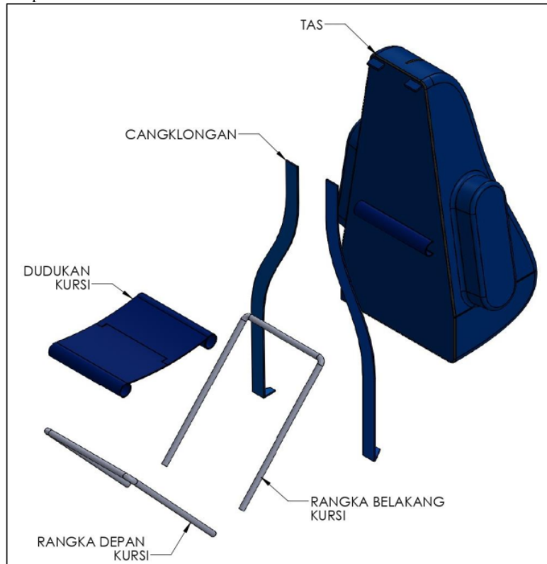
Gambar 5. Design 3D Pancing Multifungsi
