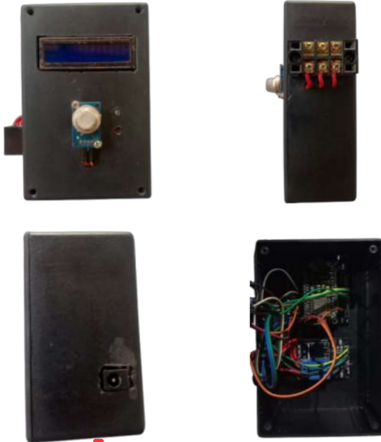
1 Gambar 4 Rangkaian Monitoring Kadar Amonia dan Pengendali Aerator Berbasis IoT
