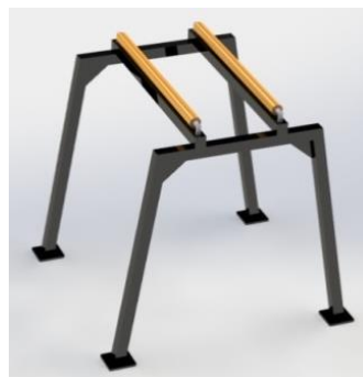
Gambar 3.3 Desain Conveyor Manual
