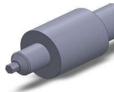
Gambar 2. Dimensi Tool FSW Geometri Hexagonal
