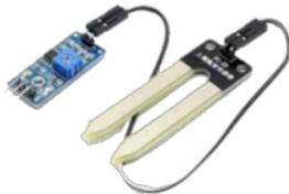
Gambar 3. Sensor Soil Moisture
