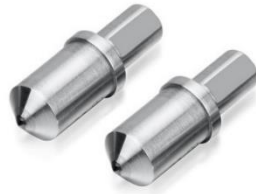
Gambar 21. Indentor piramid Diameter
