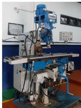
Gambar 7. Mesin Frais Universal
